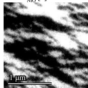
**Figure 1.** SPLEEM image with in-plane magnetization of a Fe/NiO polycrystalline bilayer with  $d_{\text{NiO}} = 20$  nm at  $d_{\text{Fe}} = 5$  nm.
