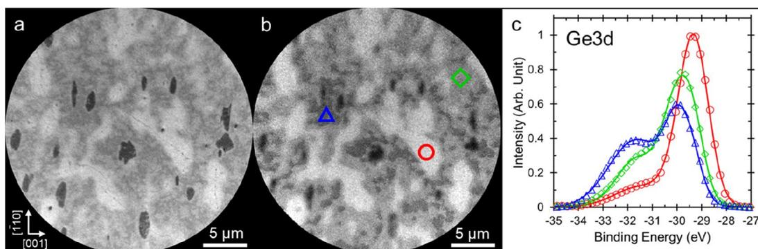
**Figure 1.** Real space distributions of germanium oxide species in graphene/Ge(110) following ambient exposure. (a) Bright field LEEM image at energy  $E = 2.5$  eV. (b) Isochromatic corrected PEEM Ge3d image at binding energy  $BE = 29.5$  eV with incident photon energy  $h\nu = 111$  eV. B (○), D1 (◇) and D2 (△) domains and spectra are indicated in (b) and (c). (c) Corresponding domain-resolved Ge 3d XPS spectra from the labelled areas in (b).
